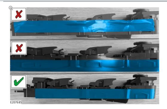
Correct position ( $\checkmark$ ) of the sealing tape.
