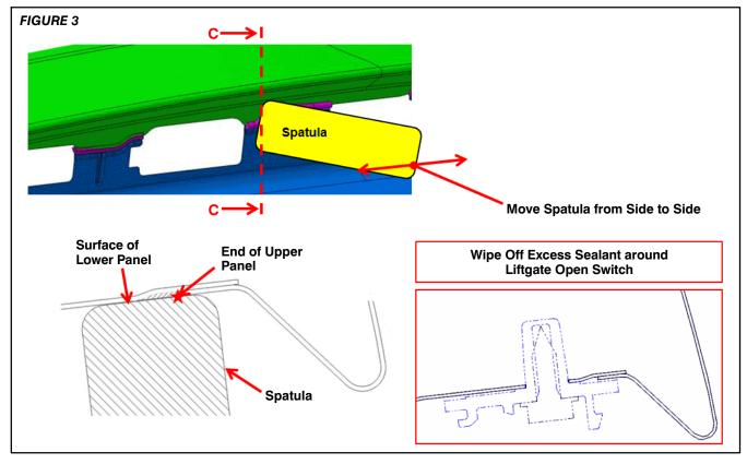
5. Using a spatula, wipe off excess sealant on the edge of the upper panel and surface of the lower panel. Wipe off any sealant on the edge of the hole for the liftgate open switch.
