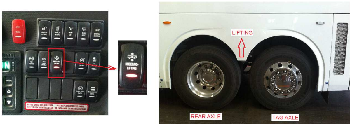
Figure -1: Kneeling/lifting operation
