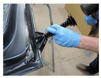
**14.** Close the hem flange using the flange closing tool.
