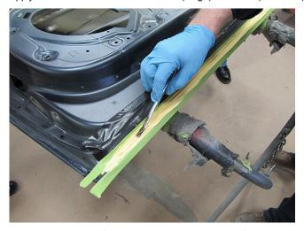
Use a small brush to finish the area, the sealer will self level to remove any brush marks.
