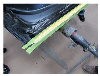
**16.** Apply a bead of \*LORD Fusor® 806HD (beige) = 10.5 oz (310.5 mL) or the equivalent, as shown to completely seal the hem flange.
