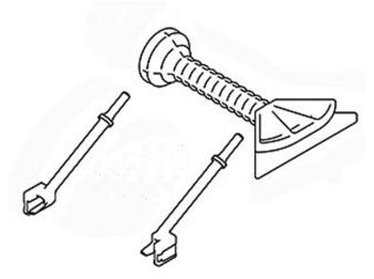
In the event that hem flange corrosion becomes a concern on lower door panels, a new tool has been released by Kent Moore, J-46162-A, which allows for easier opening and closing of the hem flange. This kit includes a left and right hand flange opening tool that is used with an air hammer, and a hem flange closir tool. Using these tools the lower door hem flange can be opened, the rust treated and the hem flange closed without having to refinish the outer door area.
