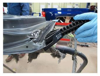
• Make an initial pass with the tool parallel to the door outer panel.
