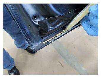
**12.** Using a small tip opening, apply a small bead of seam sealer such as \*LORD Fusor® 806HD (beige) = 10.5 oz (310.5 mL) or the equivalent to the open joint area.
