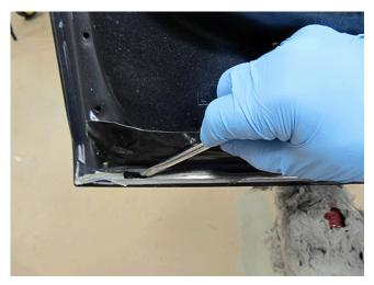
7. Using \*Lloyd's Pure Prep™ Metal Surface Preparation P/N 25418 (10 fluid ounce bottle) in a spray bottle, saturate the complete flange area with the pre diluted solution and scrub the area well, rendering a foaming of the Pure Prep.™ This will greatly improve adhesion and corrosion resistance in the repair areas.
