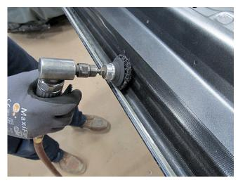
If sand blasting is not available, remove the rust using a 3-M Scotch-Brite™Clean and Strip Disc, Part # 07466, abrasive wheel.
