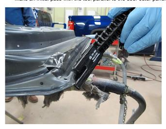
• Make a second pass with the tool at a 40° angle towards the inner panel to close the flange completely.
