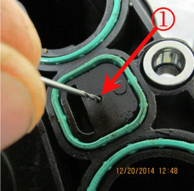
1. PCV orifice in the intake manifold
