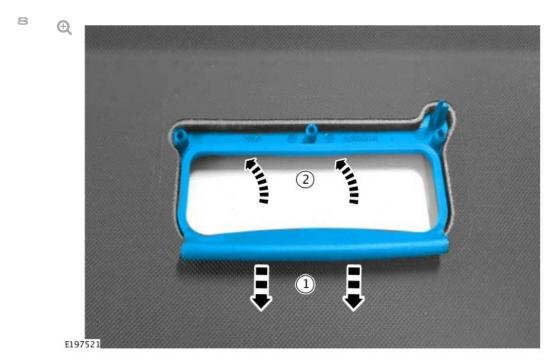
Install a new loadspace cover handle upper bezel from below.
