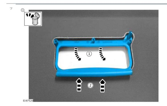
Remove and discard the loadspace cover handle upper bezel from below.
