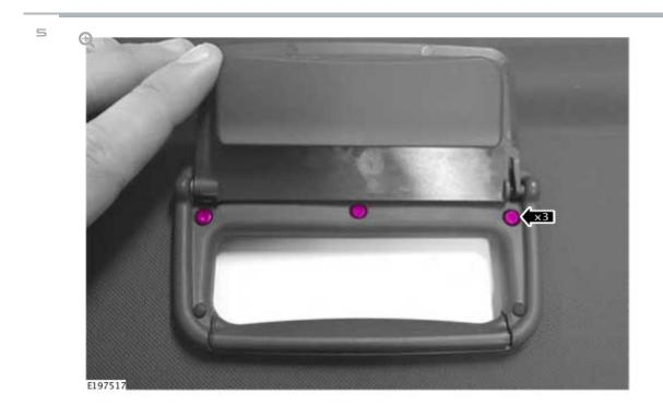
Remove the three fasteners.
