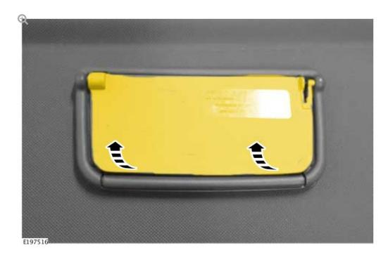
Lift the flap on the loadspace cover handle to access the fasteners.
