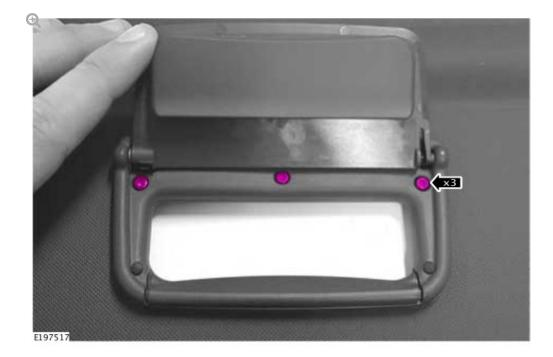
Install the three fasteners to attach the lower bezel to the upper bezel and release the flap.
