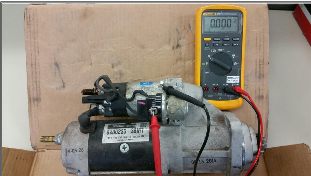
Figure 1: Starter IMS S terminal DVOM Hookup Location
