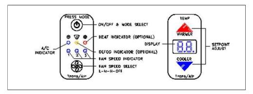
The EC4.0 climate control system has two driver control modules: Mode/Fan control switch and Thermostat. The Mode/Fan control switch turns system on/off and controls evaporator blower speed. The Thermostat displays cabin air temperature, fault and service codes, and adjusts set point temperature.
