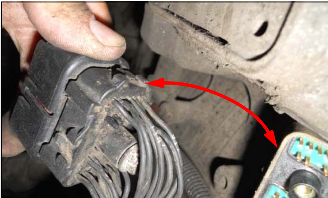
Figure 5. Transmission harness connector removed from the interface port.
