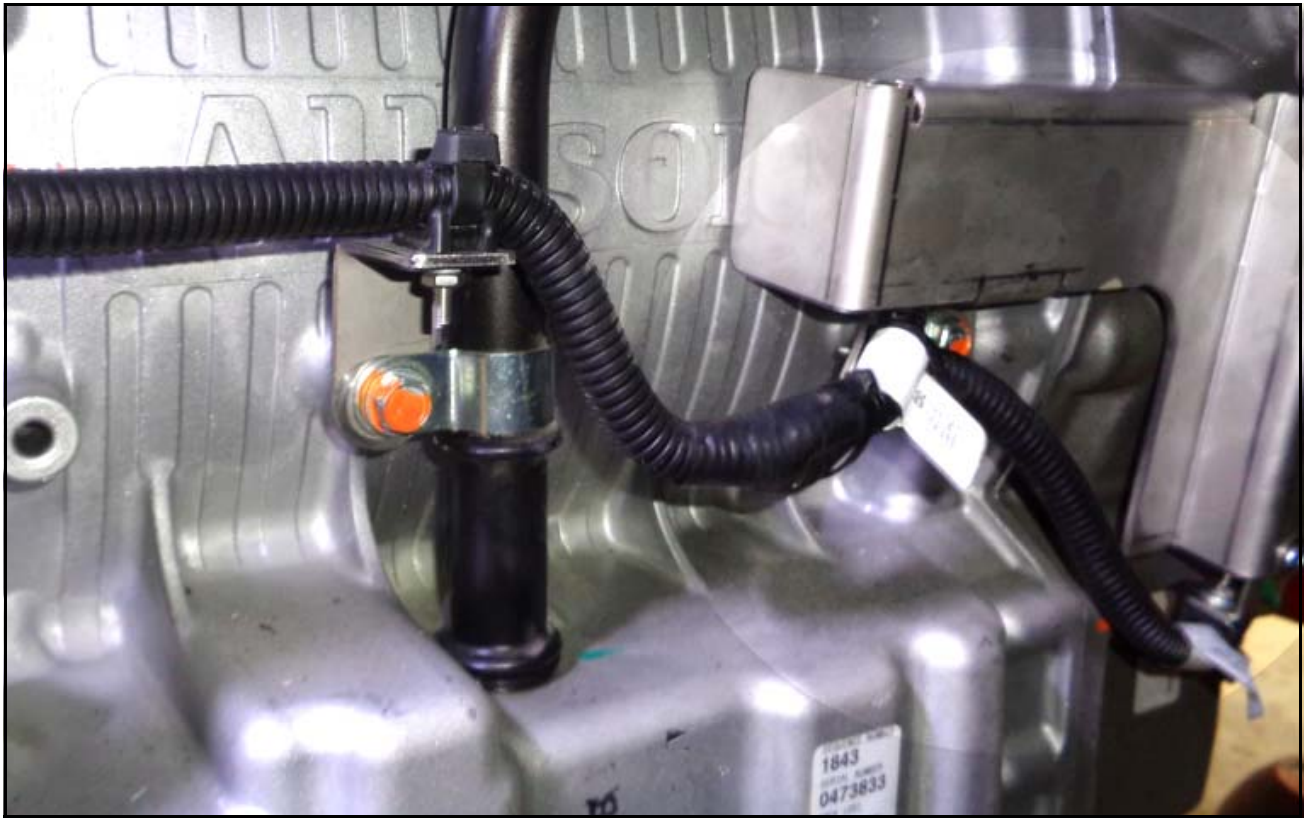
Figure 21. Transmission harness routing on protection shield.
