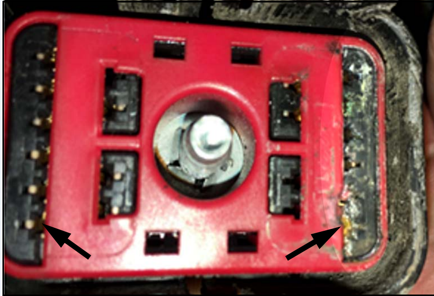
Figure 6. Evidence of corrosion on the transmission harness connector pins.
