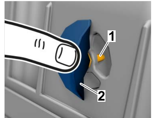
Fastening pins for water drain valves
