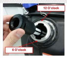
5. Reinstall the DEF tank filler cap.
