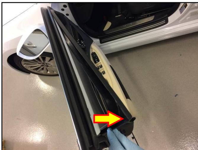
3. To remove the door panel, gently pull the door trim cover away from the door frame. Start with the top right hand corner.
