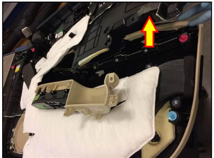
7. Use a Phillips screwdriver and remove the DDM mounting screws.
