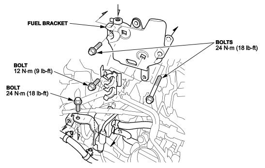
2. Remove the EVAP canister purge valve.
