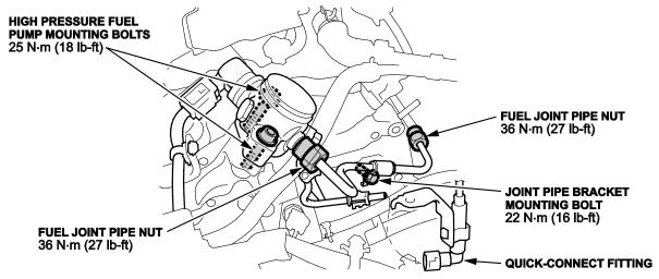
11. Reinstall the parts in reverse order, then check for any fuel leaks.
