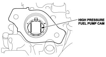
7. Set the No. 1 piston at top dead center (TDC), then rotate the crankshaft 105° counterclockwise. Check the position of the cam that drives the high pressure pump as shown. If the cam position is not correct, continue turning the camshaft until it is.
