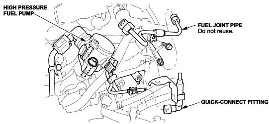
Remove the high pressure fuel pump.
