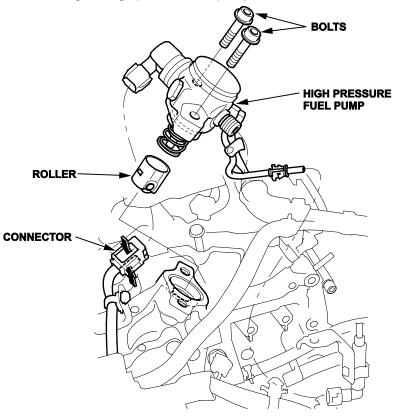
6. Rotate the crankshaft and check the high pressure fuel pump cam for any pitting, scoring, or excessive wear. If needed, replace the camshaft.
