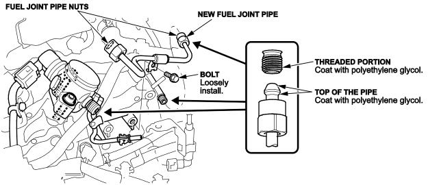
10. Torque the high pressure fuel pump mounting bolts and fuel joint pipe nuts to the specifications shown below.
