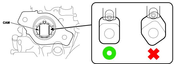
8. Lubricate the cam and roller, then install the high pressure fuel pump with the new fuel line clip. Loosely install the bolts because it will be easier to install the new fuel joint pipe.
