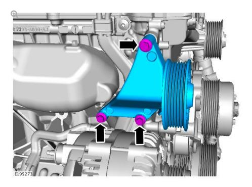
Remove and discard the idler pulley and bracket assembly.
