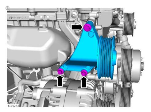
Install the new idler pulley and bracket assembly.
