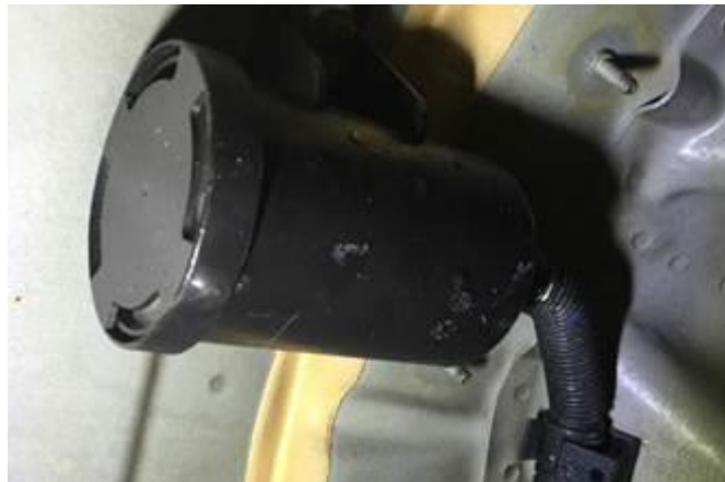
Figure 1. Ventilation tube of the activated charcoal filter.
