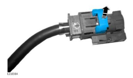
Use a suitable tool to remove the locking tab from the electrical connector at each end of the new USB link lead.
