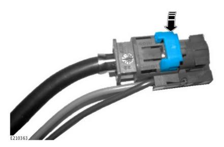
Install the locking tabs into the electrical connector at each end of the new link lead.
