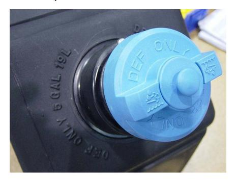
2) Grip the cap and turn counter clockwise unit the cap stops turning.
