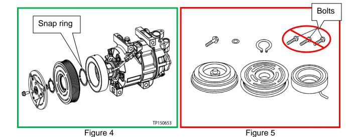
**NOTE:** The magnet coil, snap rings and bolt come with the CLUTCH COIL ASSY-COMPRESSOR (see **PARTS INFORMATION**).
