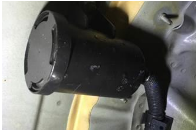
Figure 1. Ventilation tube of the activated charcoal filter.
