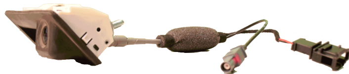
Figure 5. Completed reverse camera assembly with new electrical harness.
