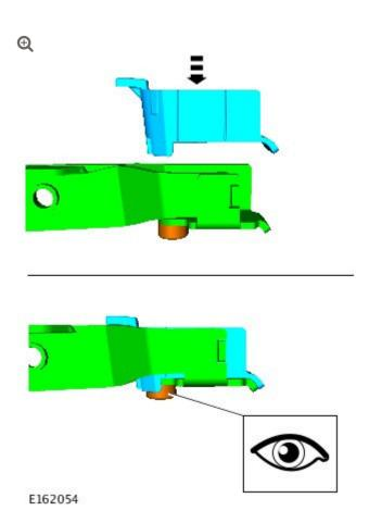
Install the insert into the roof opening panel regulator arm as shown.
