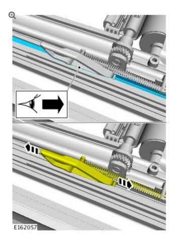
Move the locking arm back and forth to distribute the lubricating oil (C2D40864).
