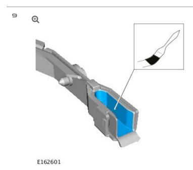
Using a suitable small brush, lubricate the insert with grease (C2D40865).
