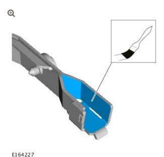
Using a suitable small brush, lubricate the opening roof panel regulator arm with grease (C2D40865).
