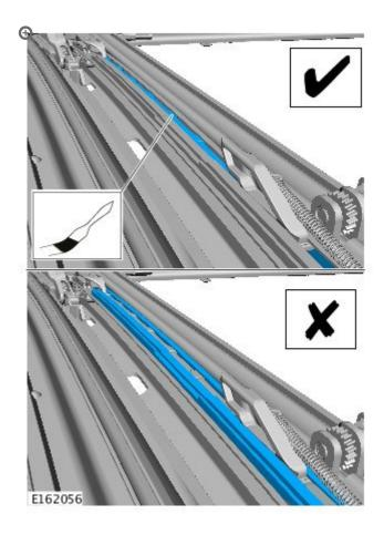
Lubricate the roof opening panel slider channel with the recommended oil (C2D40864).
