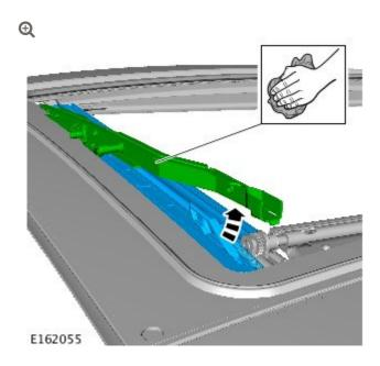
Raise the roof opening panel regulator arms into the vent position and clean them with a suitable cloth.
