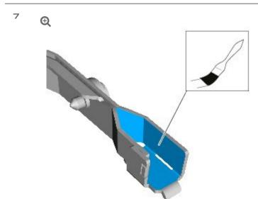
Using a suitable small brush, lubricate the opening roof panel regulator arm with grease (C2D40865).
