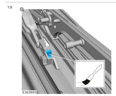
Using a suitable brush, lubricate the contact point with grease (C2D40865).
