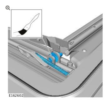
Using a suitable brush, lubricate the area shown with grease (C2D40865).
