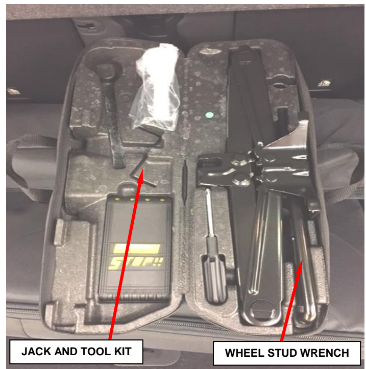
Figure 2 – Wheel Stud Wrench (2016 Model Year Jeep Renegade Shown)
