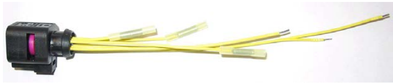
Figure 4. Crimp connectors installed on wire ends.
