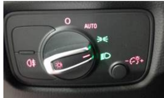
Figure 1. A headlight switch in an intermediate position.
