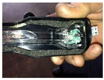
**Figure 10.** Turn signal lamp with sealing foam tape installed.
