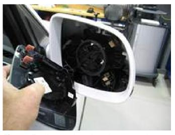
Figure 1. Exterior rear view mirror glass removed.
