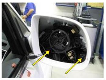
Figure 3. Location of the retaining clips.
