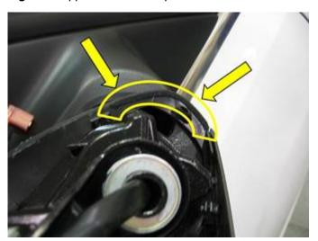
Figure 7. Felt tape applied.
