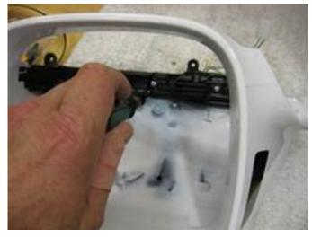
Figure 8. Removing the turn signal lamp.
