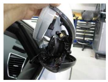
Figure 4. Removing the mirror cover.
