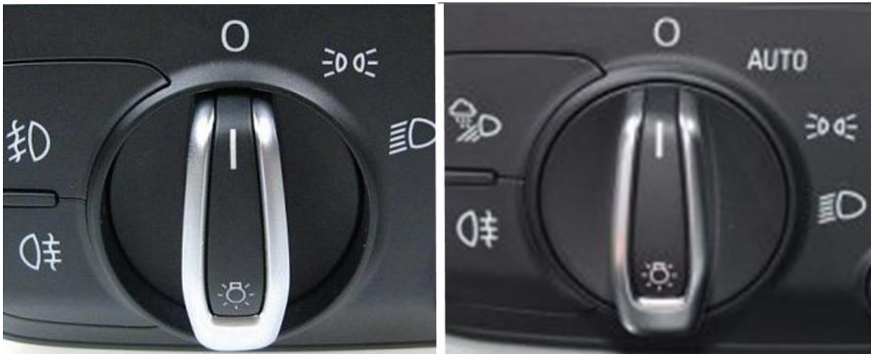
Figure 2. A3 headlight switch knob pushed in (left) and in normal position (right).
