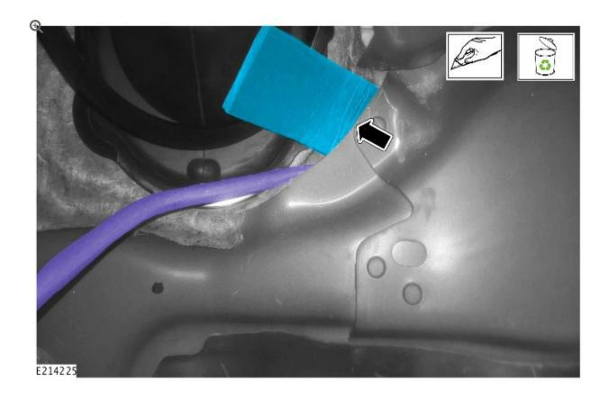
Cut and discard the excess hard foam visible from between the body panels.
