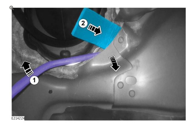
Using a suitable tool, separate the 2 body panels (1) and then install the foam pad (2) as far into the gap as possible.
