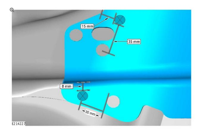
Drill 2 (two) 7mm holes and install 2 rivets in the area shown.
