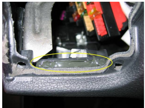
Figure 8. Additional bonder applied to top of holder.
