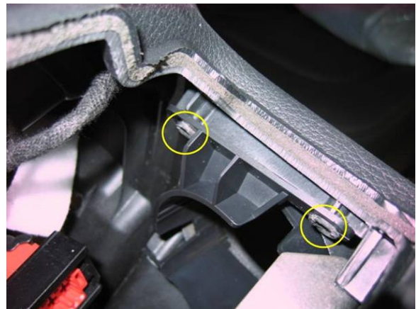
Figure 2. The broken plastic rivets, viewed from above.
