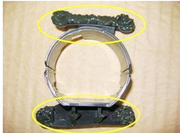
Figure 5. Attachment points after applying bonder.
