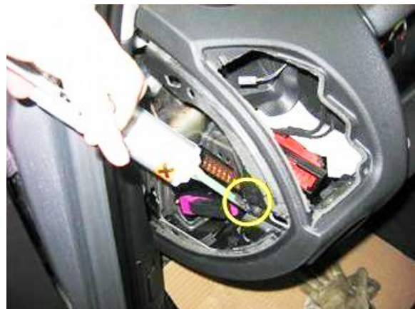
Figure 6. Applying additional bonder to four fastening points on holder.
