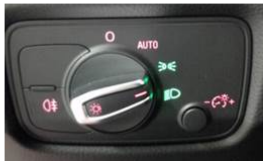
Figure 1. A headlight switch in an intermediate position.
