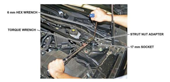
3. Remove the loose self-locking nut(s), install new a self-locking nut(s) and torque them to **44 N·m (32 ft-lb)** using a 6mm hex wrench, 17mm socket, strut nut adapter, and a torque wrench.
