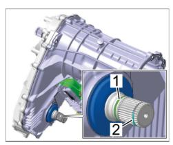
Installing O-ring and circlip
