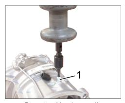
Removing old vent connection
