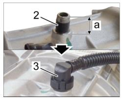
Installing new vent connection
