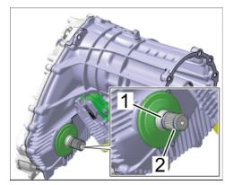
Removing O-ring and circlip
