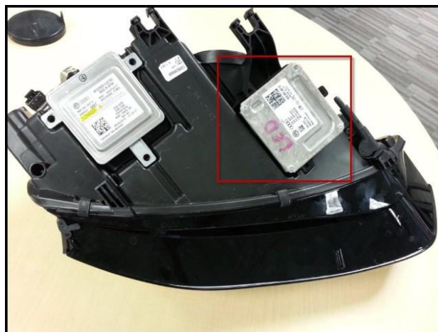
Figure 3. Daytime Running Lamp and Parking Lamp control module (DRL control module), J860/J861
