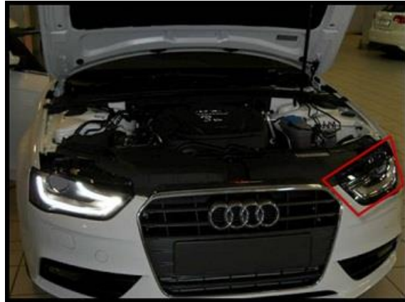
Figure 1. Driver's side LED DRL inoperative.
