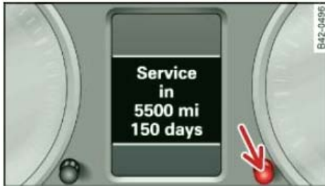
Fig. 19 Section of instrument cluster: Service interval display
