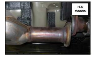
• Remove the nuts holding the front exhaust pipe onto the cylinder heads. Retain these nuts for use at reassembly.
