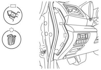
• Remove the data link connector, release the 3 retaining clips and remove the lower the instrument panel under cover.
