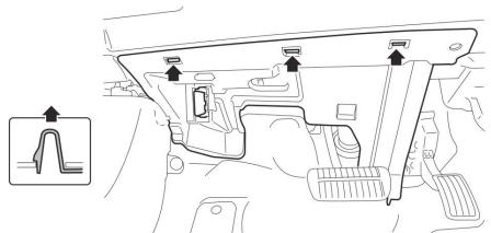
Remove the necessary screws, release the claws and disconnect the harness connectors from
