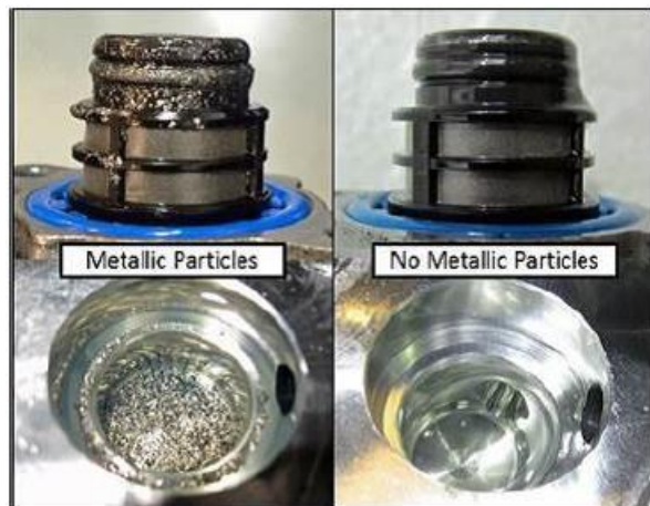
Figure 2. N290 Fuel Metering Valve and Valve Bore
