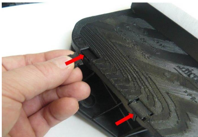
Figure 3: example Jetta: attachment of the filter housing on the air intake grille with clips part number 7L6 133 847 A (red arrows).
