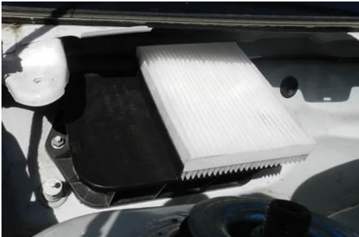
Figure 1: example Jetta: filter housing (part number 5C6 819 343). Figure 2) red arrows mark the mounting points of the clips (part number 7L6 133 847 A).
