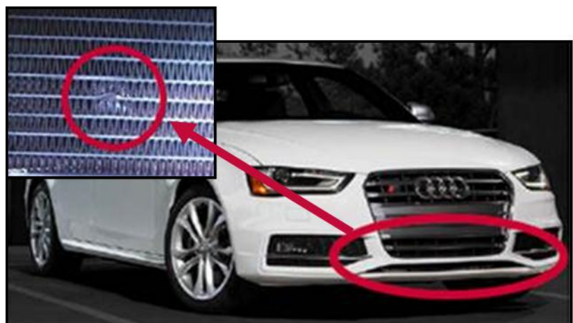
Figure 1. Damage from front-end stone impact.
