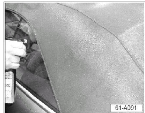
Figure 3. Applying convertible top cleaner evenly over entire vehicle.
