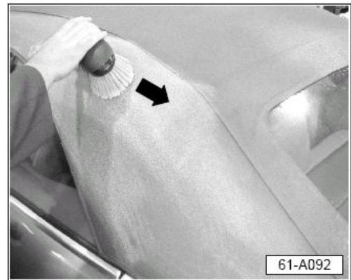
Figure 4. Using soft-bristled brush to brush in direction of fabric weave.
