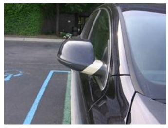
Figure 1. Tape applied to rotation collar seam.
