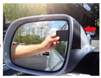
Figure 2. Tape applied over the lane change assist lens.
