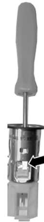
Figure 5. Retaining tabs (arrow). The socket shown is removed for clarity. Do not remove lighter socket from vehicle.
