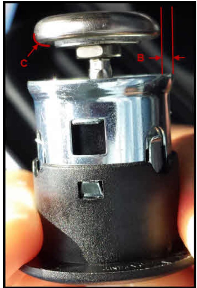
Figure 3. OEM lighter with smaller adapter head relative to lighter housing (B) and rounded edge (C).
