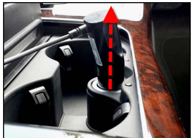
Figure 2. The arrow shows the proper angle to remove any accessory adapter.
