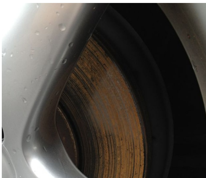
Figure 1. Disc covered with rust.
