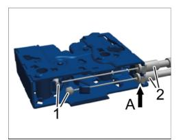
Checking front hood lock cable at the left and right
