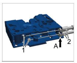
Checking front hood lock cable at the left and right
