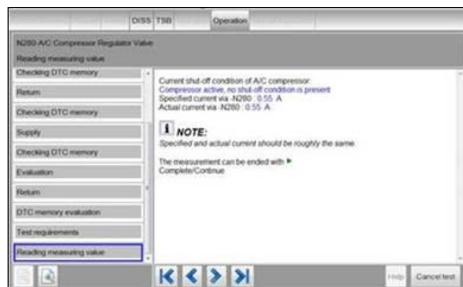
Figure 5. Checking N280 signal value Measuring Value Block.
