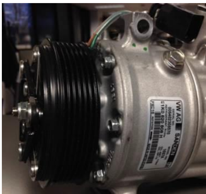
Figure 8. MY2016 AC compressor with clutch (Sanden)
