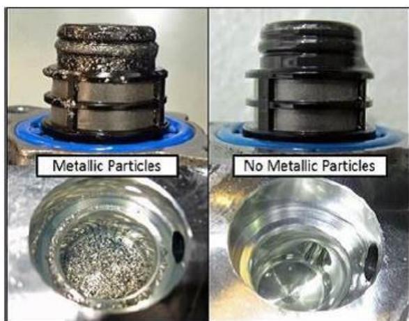
Figure 2. N290 Fuel Metering Valve and Valve Bore
