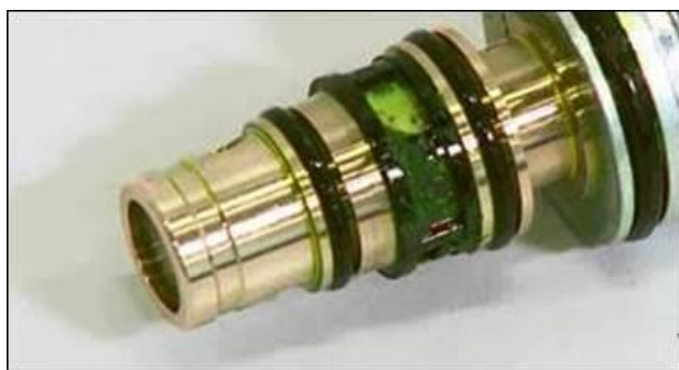
Figure 14: Severe contamination at the N280 valve filter screen.
