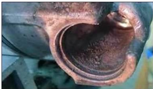
Figure 13. Corrosion in the N280 valve bore.
