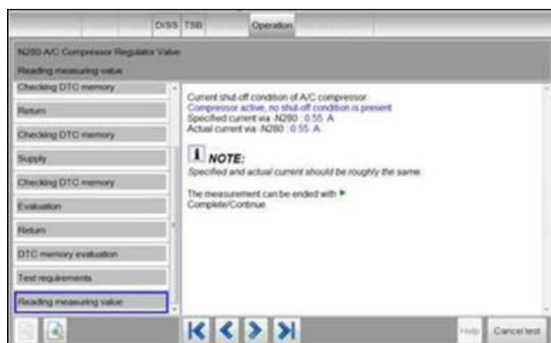
Figure 5. Checking N280 signal value Measuring Value Block.
