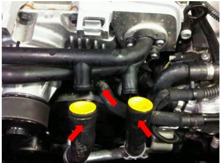
Figure 10. Coolant hoses (arrows)
