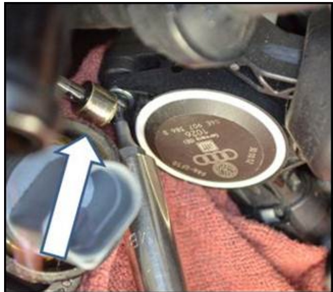
Figure 13. Use a magnet (arrow) to hold the screws during removal.
