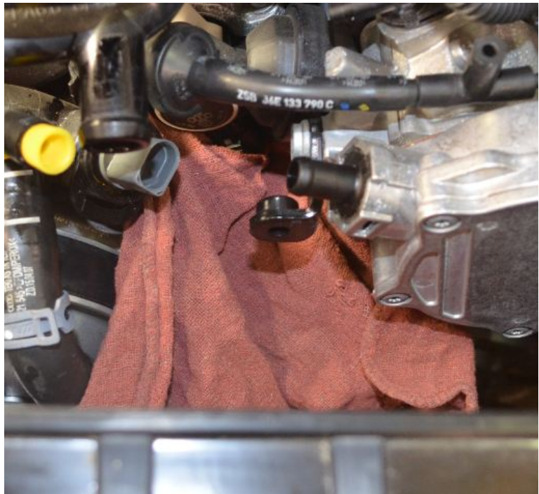
Figure 12. Place a shop rag under the screws.
