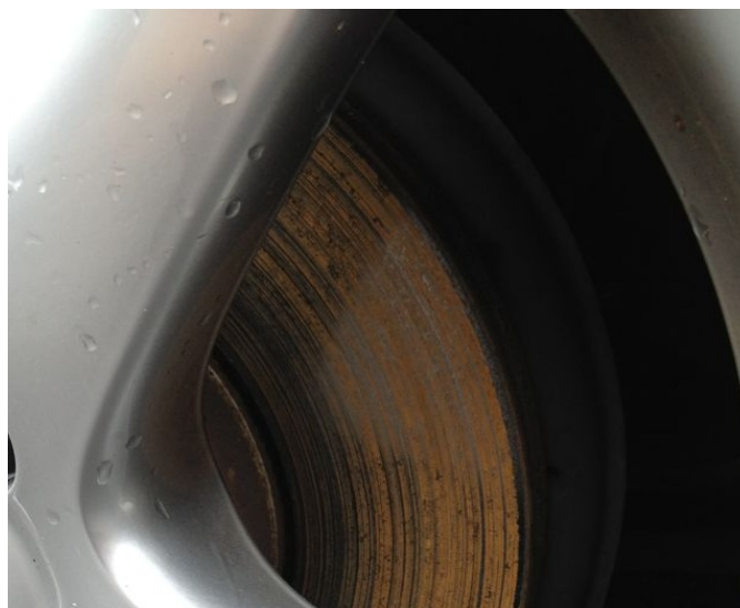
Figure 1. Disc covered with rust.
