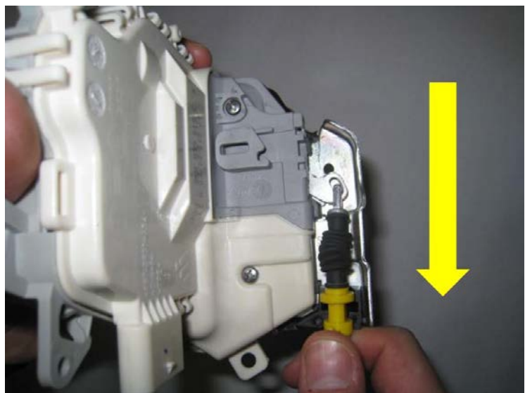
Figure 5. Pulling down the Bowden cable.
