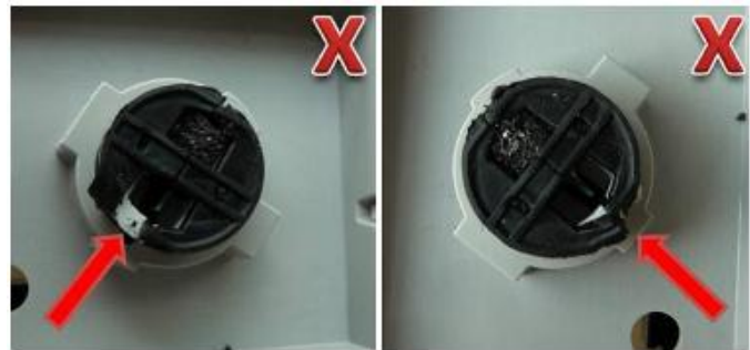
Figure 6. Examples of damaged seals
