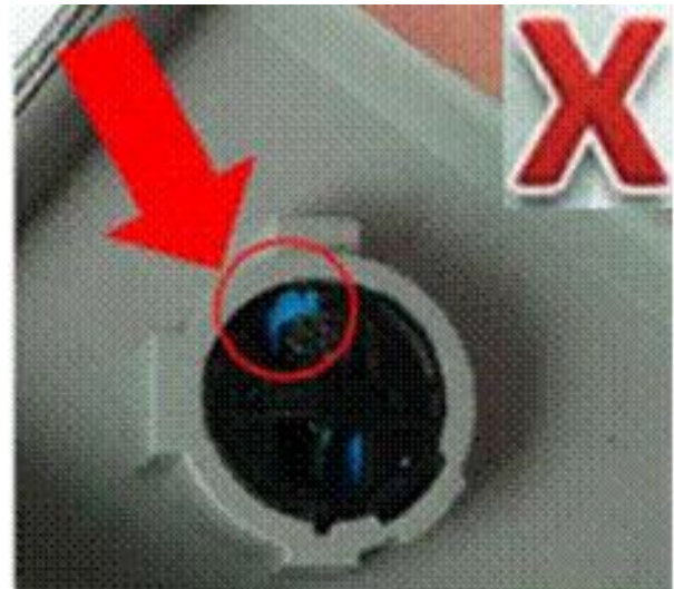
Figure 9. Damage caused by a pinched seal.
