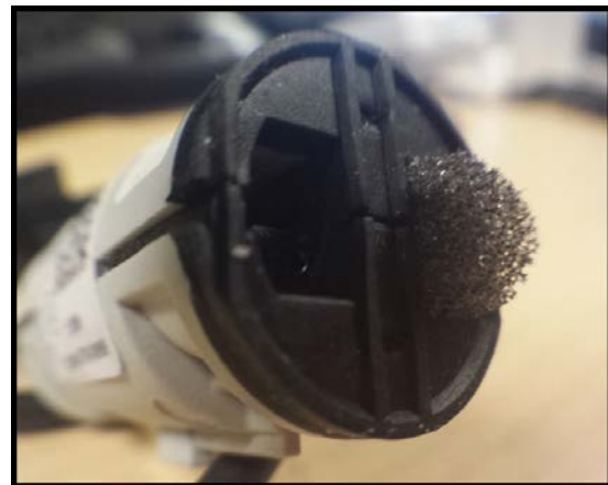
Figure 9. Foam is partially pulled out of the microphone.
