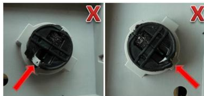
Figure 7. Examples of damaged seals
